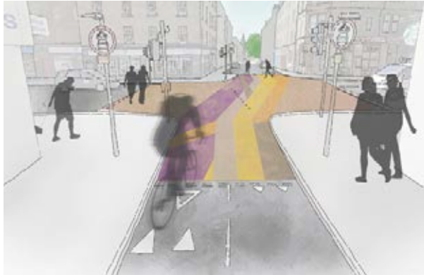
Create a level pedestrian surface for East-West and North-South movement using raised table over minor roads to prioritise pedestrian and cycle movement. This might extend super graphic painted surface from The Causey.
