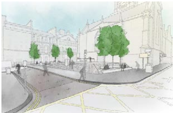
Redesign of Hunter Square to provide improved seating opportunities, shelter and soft landscape and relaying setts to give a level walking surface across Blair St.
